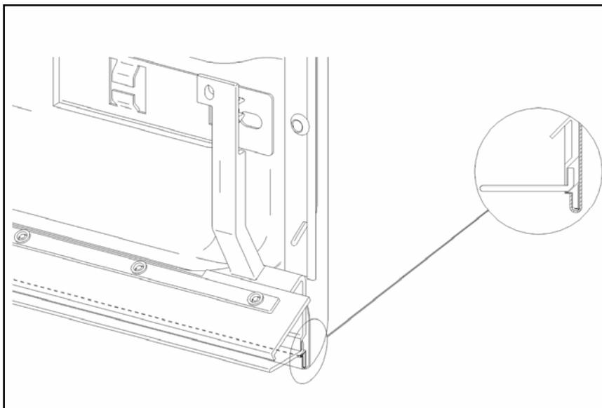
**Figure 5-13:** Lower door seal holder
