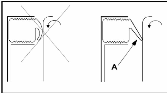
**Figure 5-14:** Door Seal with Door
