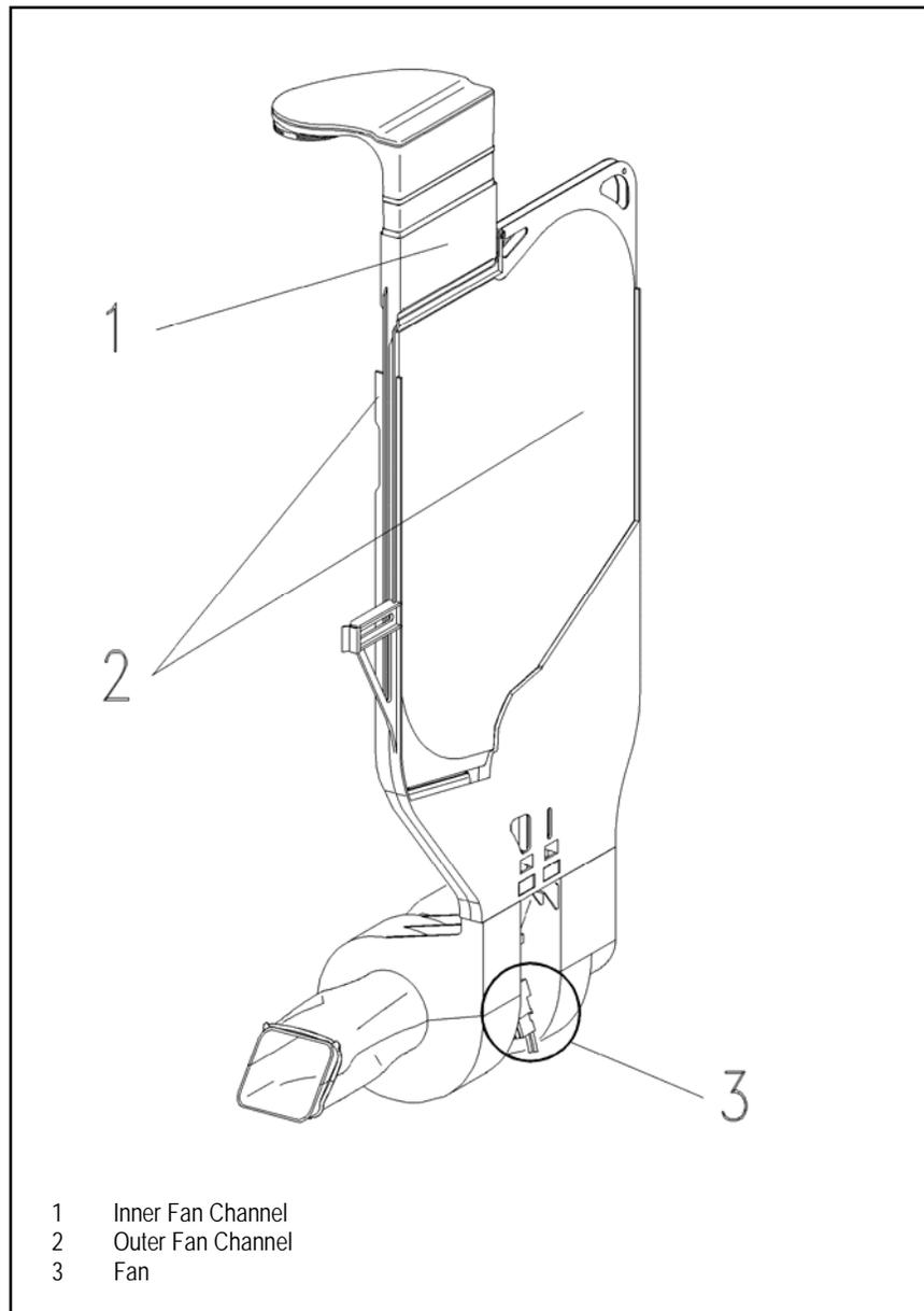
**Figure 4-17:** Drying System UTT Version 1
