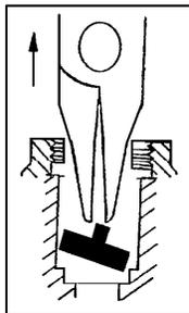
**Figure 5- 27:** Removing the Flow Restrictor.
