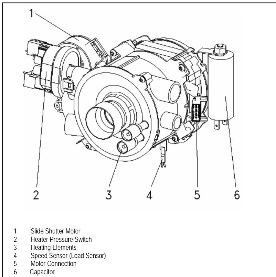
**Figure 4-10: Circulation Pump - Components**
