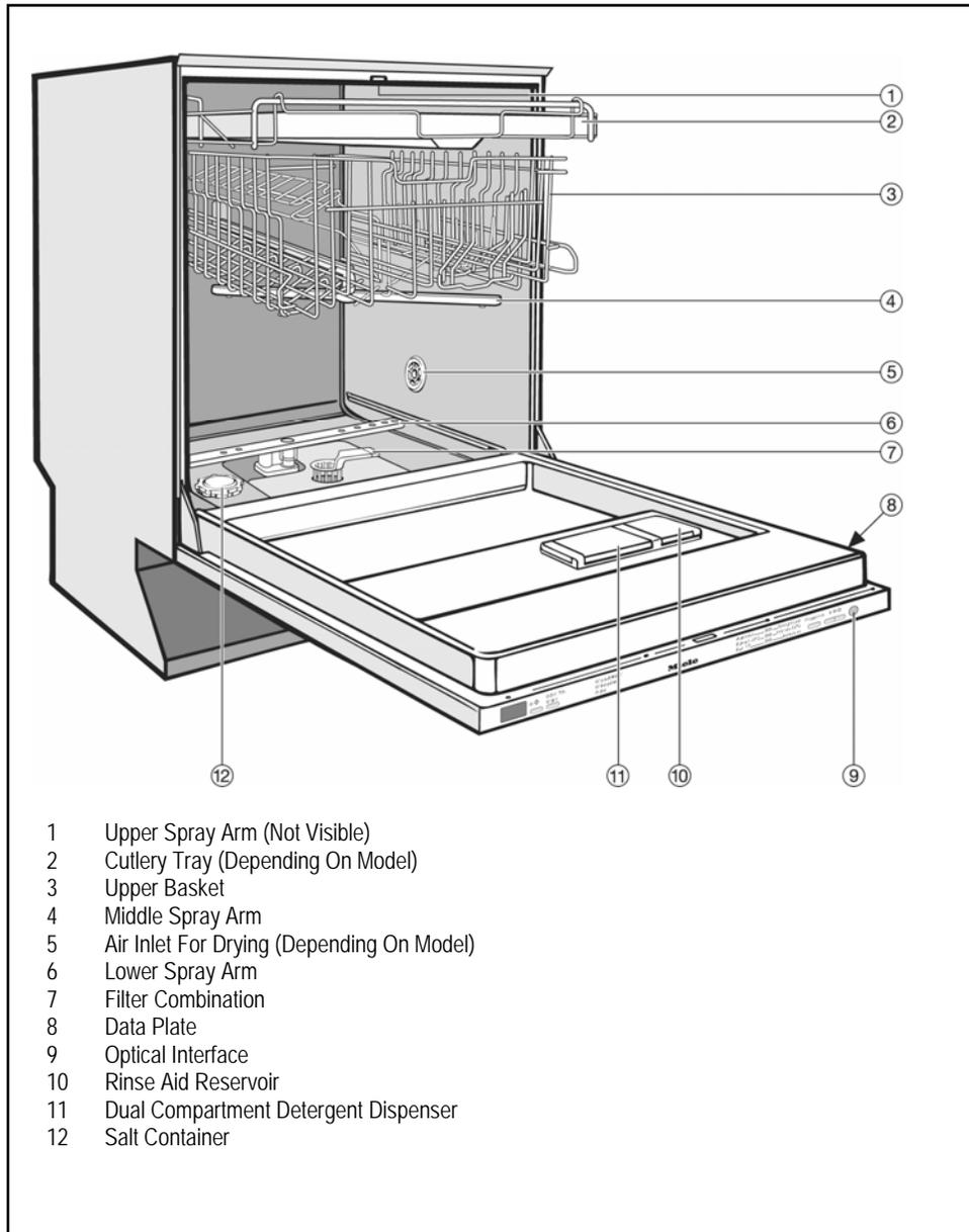
**Figure 1-2: Appliance Overview (Typical Fully Integrated (Vi) Unit)**
