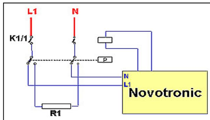
**Figure 6-7:** Circuit test path for F-51 (initial state)
